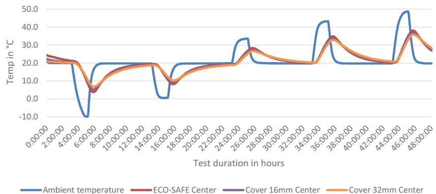
Figure 1: Results of climate chamber tests.
